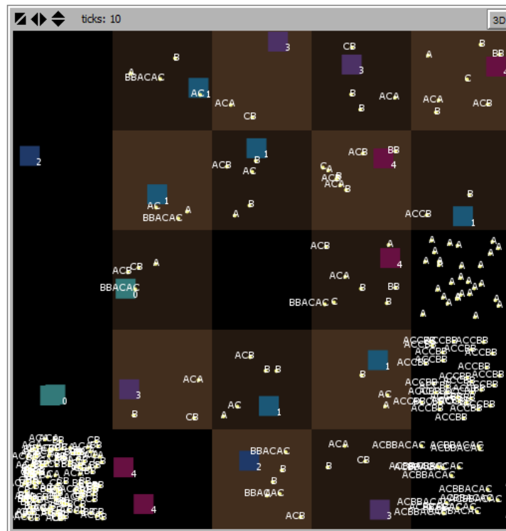
Figure 21 – The Factory Model with workers (brown patches) and machines (different coloured squares). Free machines are located in the black patches on the left. Resources are provided on the patch in the lower left corner, whereas the targets already produced are moved to the three black patches on the right. Workers keep things they are currently working on or that are by-products on their patch.
